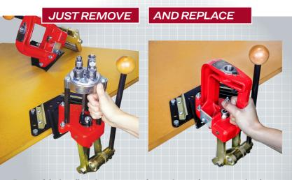
Patented design allows instant press change. So sturdy you can resize the monster 50 BMG case, then quickly switch to a smaller press for priming or other operations. Trapezoidal base block slides into perfect register and made immoveable with the quick tightening of four bolts.
